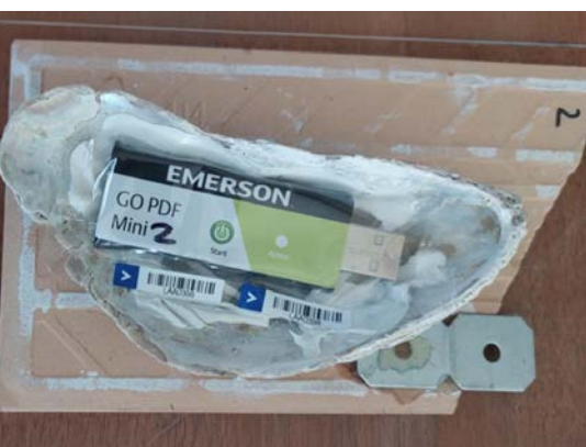
Temperature Datalogger embedded in shellfish that was installed in the mudflats
