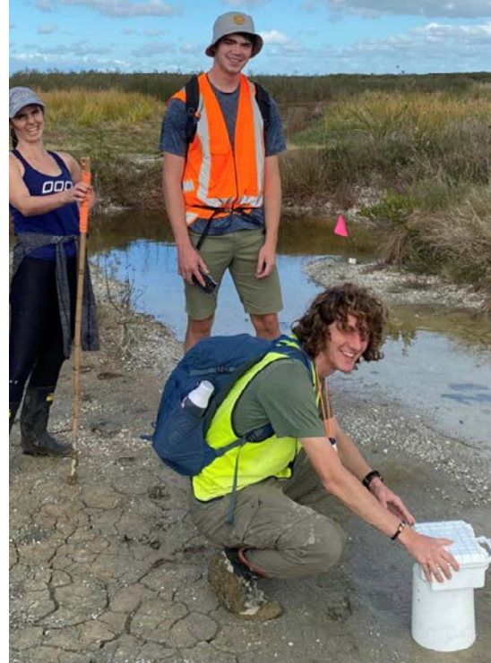
Methane monitoring using the EcoQuest methane flux meter ECOQUEST
