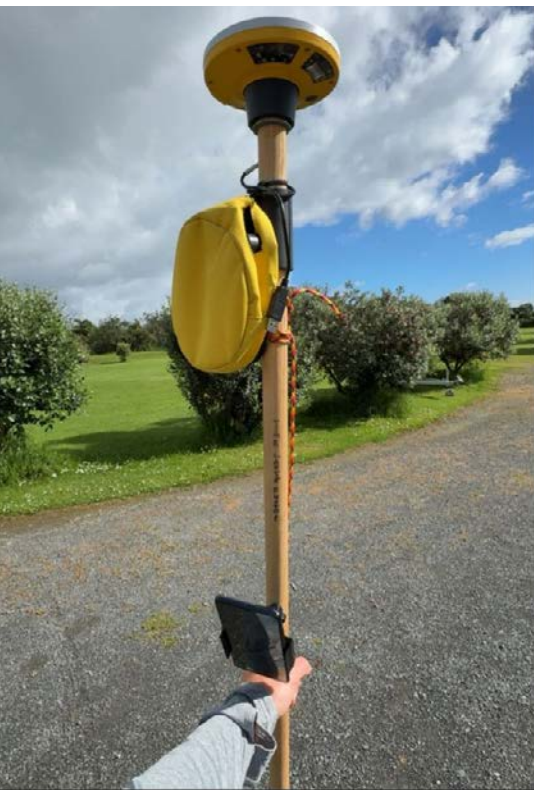
Our differential GPS antenna providing cm level accuracy in position and altitude
