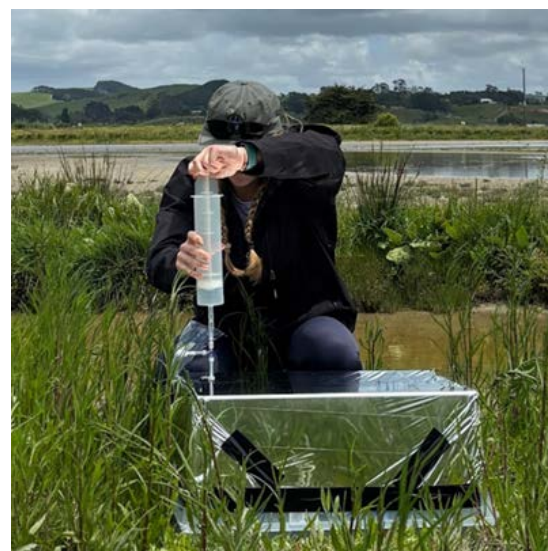
Taking gas samples in the reserve from a chamber set on to the substrate. ECOQUEST
