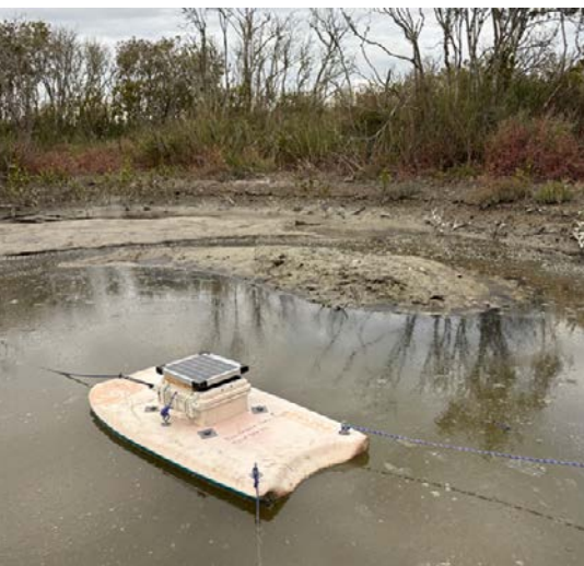
Floating automated water data logger, April 2025
